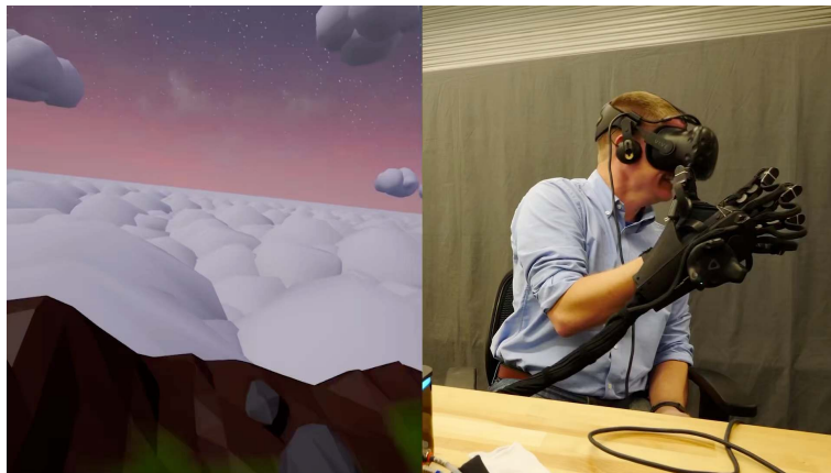
HaptX (armored exoskeleton, 100 actuators)
