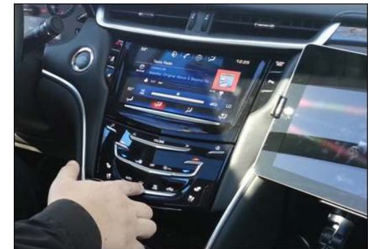
Infotainment system in car with haptic touch screen
