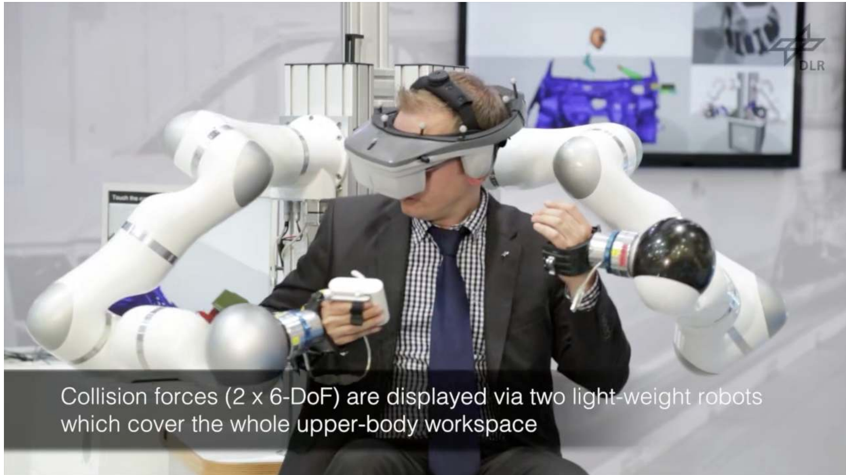
DLR: A Platform for Bimanual Virtual Assembly Training with Haptic Feedback in Large Multi-Object Environments
