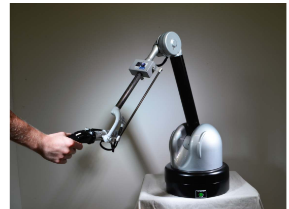
Virtuose (6 DOF's tracking, 3 DOF's force)
